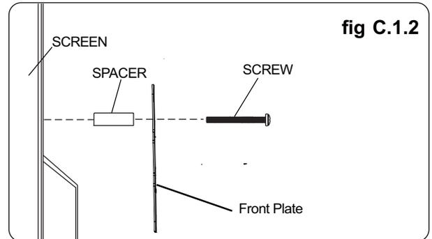
Select the small, medium, large or extra large screws from the screw package. Fastener pack then attach screen brackets(AA) to screen following figure C.1.1 or C.1.2 on page 7.
