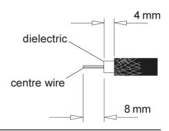
Pass the connector over the cable and twist on until the dielectric is flush with the bottom face of the connector. Approximately 2 mm of the centre wire should protrude from the connector (trim if necessary).
