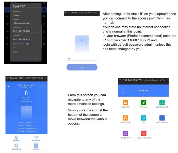
To activate the web service so that you can see the GUI setup screen you will need to set the IP on the access point to static.
