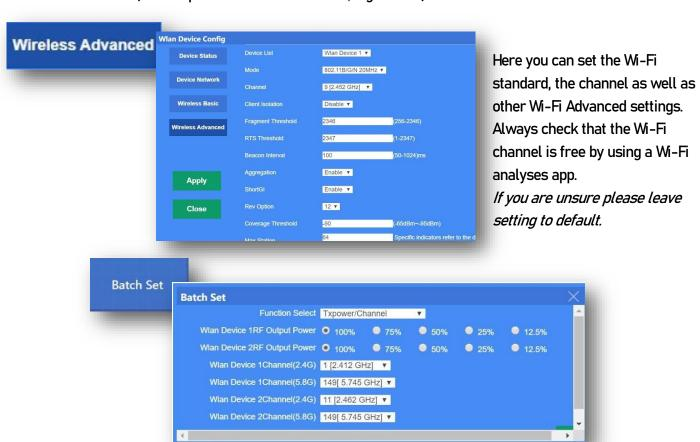
Batch set allows you to quickly select the Power output of 2.4G & 5G on each device and select the channel they will TX on all from the one page. This will be sent out to all access points connected.
