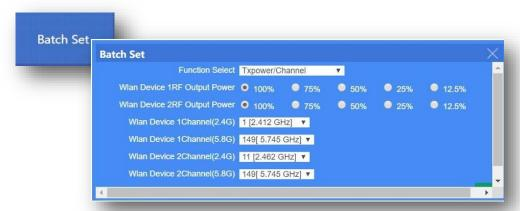
Batch set allows you to quickly select the Power output of 2.4G & 5G on each device and select the channel they will TX on all from the one page
