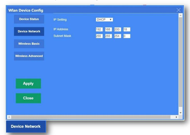
Device network:- The area where you enter the IP allocation method that you will be using for all of the Access Points that are connected to the gateway:
