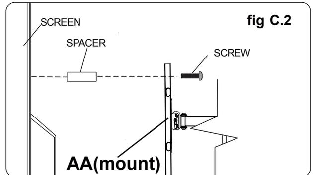
Select the small, medium, large or extra large screws from the baffled .Fastener pack then attach screen brackets(AA) to screen following figure C.1 or C.2 on page 7.
