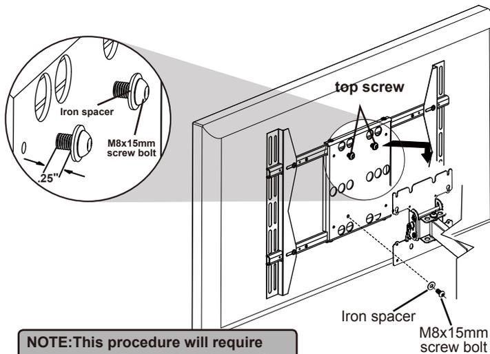
**NOTE:** This procedure will require two persons. Ensure that the arm is set to its maximum negative tilt prior to attaching the display
