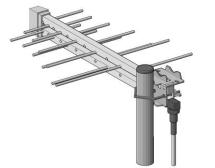
Aerial adjusted for horizontally polarised transmission
