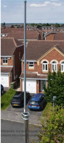
SWR on both antennas was under 1.5:1 across the frequency range measured on my NanoVNA-H4
