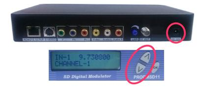
Reset to Default – Turn OFF the unit. While pressing UP and DOWN buttons at the same time, turn ON the unit. Release the UP and DOWN buttons when the LCD shows Reset To Default. The unit will reset to factory default.
