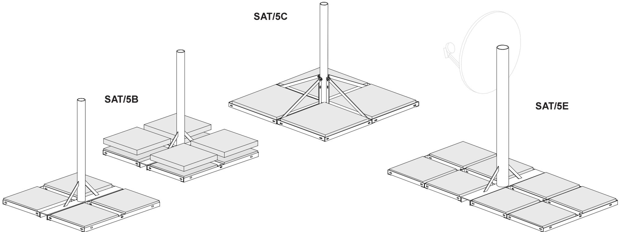
Suitable roof surfaces should be smooth, any gravel or dirt should be removed from soft roof coverings or damage and thus rain ingress may ensue due to weight of mounts. Note that extra paving flags may be used if needed.
