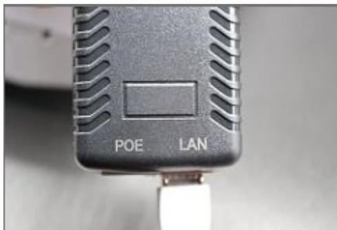
1. LAN on the PoE inject goes to the router. and POE on the PoE injector goes to the CPE.
