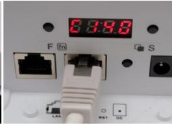
Setup is via the three buttons under the removable cover. Lift the catch and slide downwards to remove the cover and you will see two RJ45 sockets labelled LAN and WAN.
