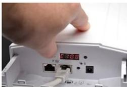
5. On the CPE connected to the router press the left "F" button and change the displayed letter C to letter "H" (Host) by using the right button labelled "S".
