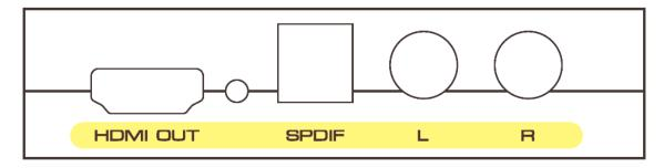
**HDMI OUT:** HDMI output interface. **GREEN LED:** HDMI output led status light.
