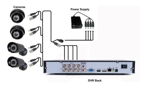
**Top Tip:** If you need to shorten the cable, use our universal BNC plug (PROCON52) as well as one of our DC plugs (PROCON70) or DC sockets (PROCON71), depending on the connection required.
