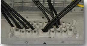
The gland plates and gaskets ensure that even after cable entry installation the glad plate and cabinet remains IP66 rated, unlike other brands. Simply make a pilot hole in the sealed gland plate underneath the cabinet and then feed the cable/s through into the cabinet. The gland plate will then seal around the cable.
