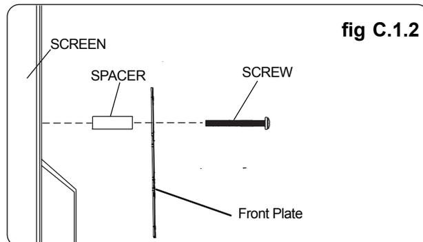
Select the small, medium, large or extra large screws from the screw package .fastener pack then attach screen brackets(AA) to screen following figure C.1.1 or C.1.2 on page 7.
